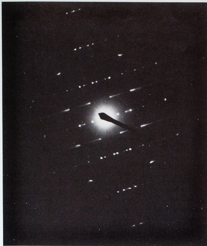
FIGURE 36-2. Selected area electron diffraction pattern of a chrysotile asbestos fiber shows the typical 0.53-nm interlayer line spacing. The prominent streaking along the layer lines is characteristic of chrysotile asbestos. (From Roggli VL, Coin PG. Mineralogy of asbestos. In: Roggli VL, Greenberg SD, Pratt PC, eds. Pathology of asbestos-associated diseases. Boston: Little, Brown and Co, 1992.)
